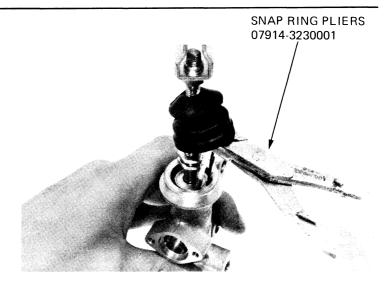
Remove the master piston, primary cup and spring.
