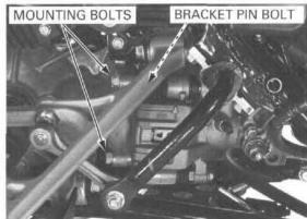
Remove the bracket pin bolt and pivot the caliper body.
