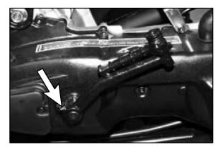
23. Carefully install the engine into the chassis. Secure the engine with the engine mounting bolts.
