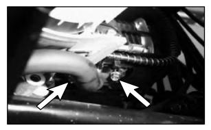
27. Install the air box and carburetor.
