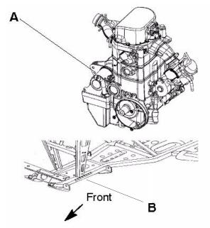
The machine model number and serial number are important for vehicle identification. The machine serial number is stamped on the lower left side of the frame tube (B).
